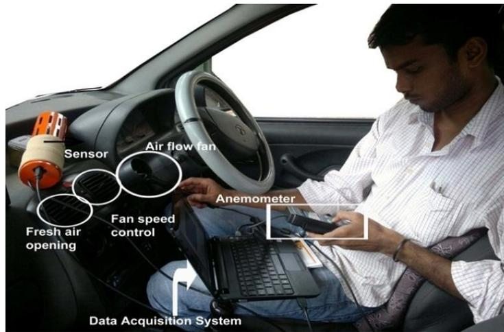
**Figure.1 Photographic image of Experimental set up**
