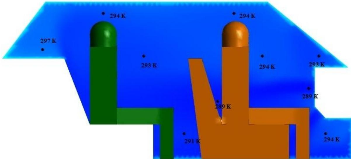
Figure.4 Temperature distributions for human load of 4
